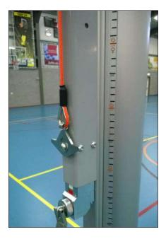
Pre-tension the net using the cable grip.
