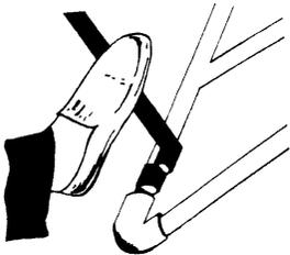
Kick out leg braces (at bottom). Note: Do not hang on end leaf. Use feet not hands when removing the leg braces.
