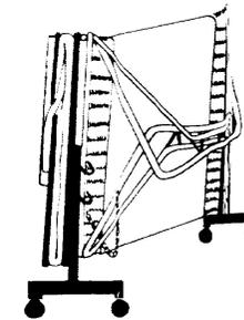
(Re-fasten hooks 101 & 99 only) and pick up rear leg and fold under front leg. Trampoline is now ready to wheel away.
