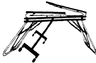
Go to opposite end of trampoline and kick out leg braces and fold end leaf over. Insert roller stands at an angle (as diagram above) into pivot point on trampoline side frame.
