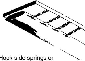
Hook side springs or Cables evenly along side rails. Do not completely finish one side before starting other, but space the work evenly to ensure equal pull.
