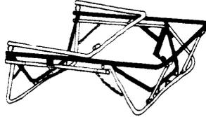
Unfold as shown in pictures 13-15 so frame rests on legs. Hook suspension system (springs or rubber cables) into frame ends only. Have hooks down on opened end of frame and up on closed end.
