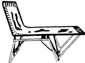
Lift and fold end rail. Note the first end leaf will be under tension and the momentum MUST be controlled at ALL times by two qualified people.
