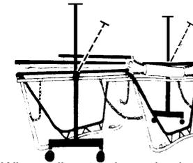
When roller stands are in place ONE person at EACH side of the trampoline is required to operate the roller stands. Before disengaging locating pin, ensure hand lever firmly held with one hand. Rotate the hand lever towards the floor and engage locating pin securely in place.
