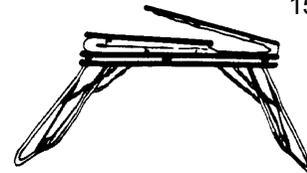
Two people to unfold one end leaf and secure by inserting leg braces into bushes on leg. Note: Do not hang on end leaf.
