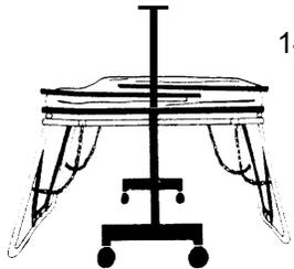
Spread leg sections. Before disengaging locating pin ensure that the hand lever is firmly held with one hand. Rotate hand lever to its OPEN position and re-engage locating pin securely in place. (SEE DRAWING 617-18 - UNFOLDING)
