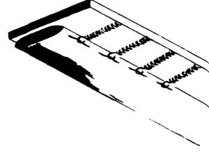
Hook side springs or cables evenly along side rails. Do not completely finish one side before starting other, but space the work evenly to ensure equal pull.
