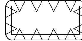
Fit twelve elevator springs interlaced with riser straps in positions shown.
