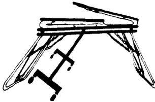
Go to opposite end of trampoline and kick out leg braces and fold end leaf over. The trampoline is now ready to attach the roller stands
