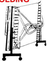
Grasp top leg and lower bottom leg to floor, rotating frame. Unfasten karabiner hooks on both chains of the top leg and push down on leg below hinge. This allows opposite leg to swing through, re-fasten chains.
