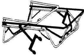
Unfold as shown in pictures 12-15 so frame rests on legs. Hook suspension system (springs or rubber cables) into frame ends only. Have hooks down on opened end of frame and up on closed end.
