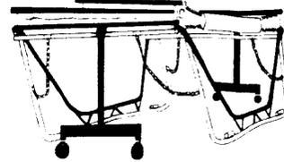
(Unfasten karabiner hooks on both chains 101 & 99 only) and place hands on bed and push forward. Trampoline will roll along floor allowing rear leg to fold under, use front leg to control movement.
