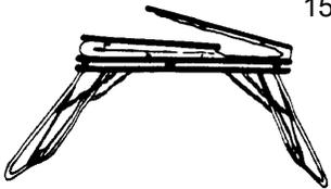
Remove roller stands. Pull leg sections (below the chain) Two people to unfold one end leaf and secure by inserting leg braces into bushes on leg. Note: Do not hang on end leaf. Use feet not hands when locating the leg braces.
