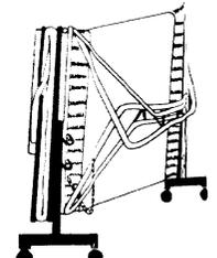
Unclip karabiner hooks on chains of end folded last and push leg below hinges, to allow opposite leg to rotate underneath. Re-fasten chains. Pick up lower leg and fold under top leg rotating trampoline into the vertical position.
