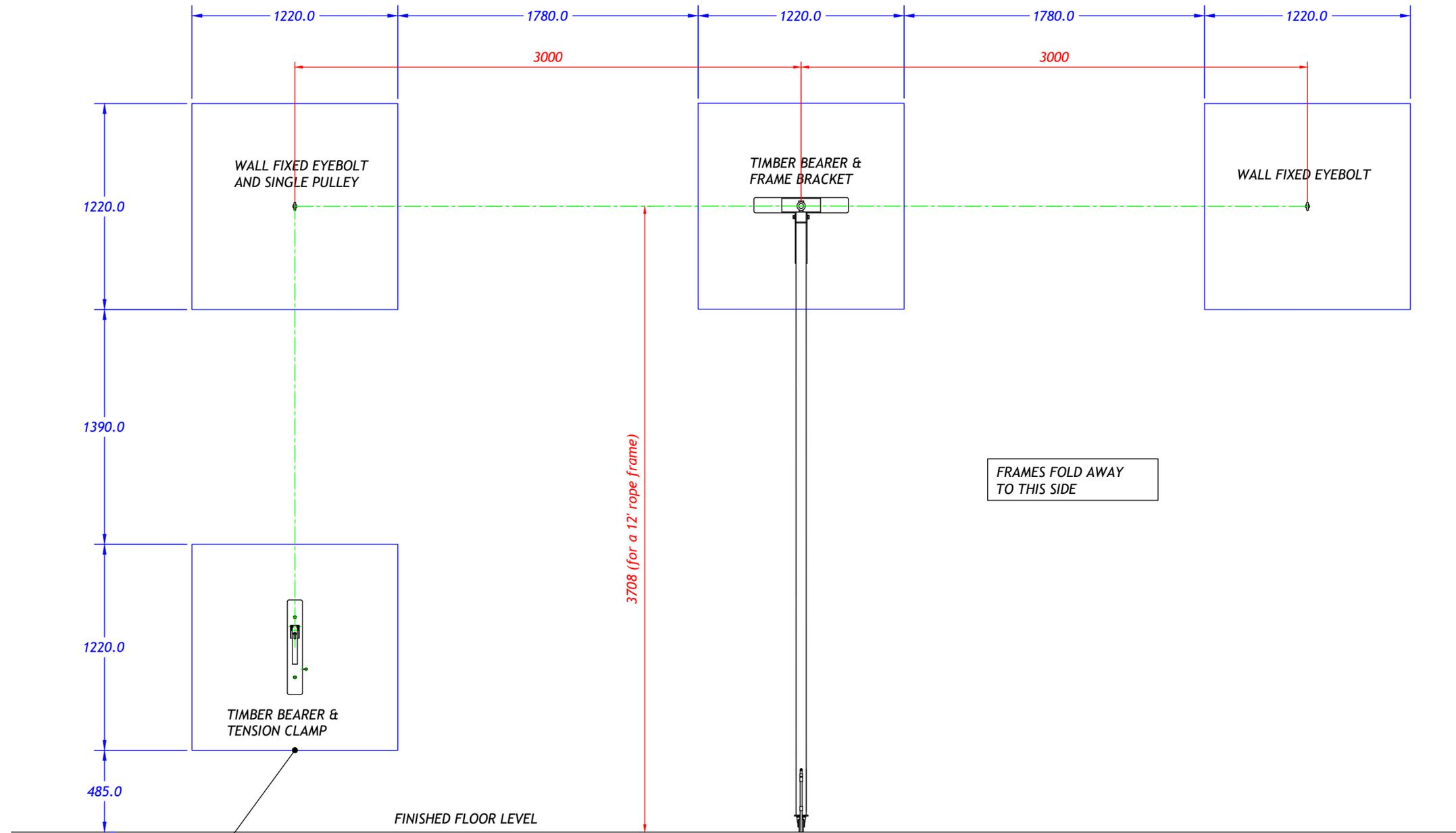
4no blue rectangles indicate plywood to walls to accommodate frame fixings. Minimum 18mm thk pattress can be surface mounted or between studs.
