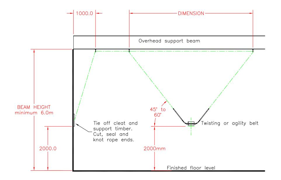
D: S.McL, 28/07/06, CSP2-2064. Minimum height 6.0m was 5.5m — Change due to revised British Standard-1892 C: TJH, 12/01/01, CSP2-1477. REDRAWN ON C.A.D. WITH MINOR UPDATED CHANGES.
