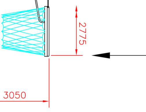
Wall / steel is to be capable of accepting 190kgs (this includes a 90kgs person hanging on to the ring)
