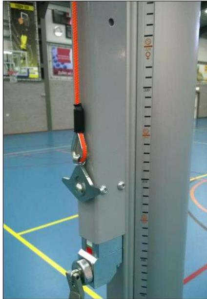
Pre-tension the net using the cable grip.
