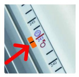
**NOTE**: The height indication on the post is not the height measured from the floor. This height indication on the post together with the orange stickers on the sliding strip is an assist for the adjustment of future setups. (Assuming that the same combination of floor sockets and posts are used)
