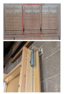
The stage unit will start to lower under its own weight. The integral gas struts lessen the weight and assist the lowering of the unit. Person 1 and 2 MUST take the weight as the frame lowers – the gas struts are to assist and not to take the entire load.
