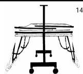
Spread leg sections. Before disengaging locating pin ensure that the hand lever is firmly held with one hand. Rotate hand lever to it's extended position and re-engage locating pin securely in place.
