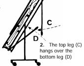
When transporting to another building or over rough ground, it is best to strap the legs in place and to strap the roller stands to the frame. Never bump up and down steps.
