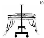
Place roller stand hand lever in extended position making sure the locating pin is engaged securely in place. Raise securing arm to uppermost position and locate roller stand pivot pin into socket on trampoline side rail.
